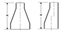
ASME B16.9 A234 WPB BW Eccentric Carbon Steel Pipe Fitting Large-Caliber Reducer
