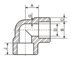
ASTM A105 90 Degree Socket Weld Forged High Press Elbow
