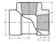
Forged ASME B16.11pipe Fitting 3000# Screwed High Pressure Tee
