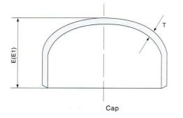
A234wpb ANSI B16.9 Seamless Butt Weld Carbon Steel Special Pipeline Cap
