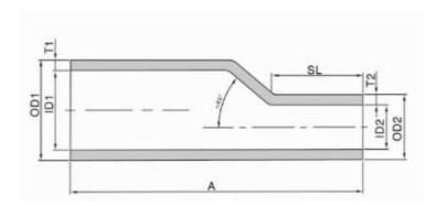
Mss-Sp-95 Stainless Steel A182 Eccenthic Swaged High Press Nipple
