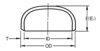
DN80 Sch40 Pipe Fitting Carbon Steel Large-Caliber Cap
