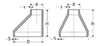
ASTM A234wpb Butt Welding Carbon Steel Special Pipe Fitting Reducer
