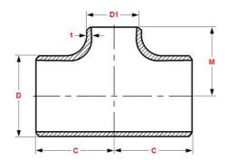
ANSI B16.9 ASTM A234wpb Butt Welding Smls Special Pipe Fitting Tee
