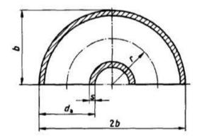
ASME B16.9 3D 5D 12D Special pipeline Carbon Steel Pipe Fitting Bend
