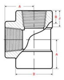
3000lbs Carbon Steel Forged Pipe Fitting Thread Tee High Press Pipeline
