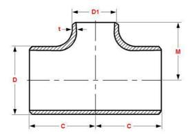
ASME B16.9 304/304LButt Weld Stainless Steel Special Pipe Fitting Tee
