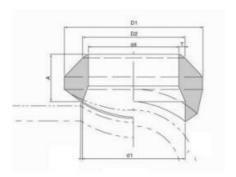
3000# Forged Socket Pipe Fitting High Pressure Weld Outlet
