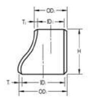
ASME B16.9 Stainless Steel Eccentric Pipe Fitting Large-caliber Reducer
