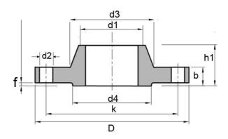
ANSI Class 300 F304 Carbon Steel Forged Threaded Flange
