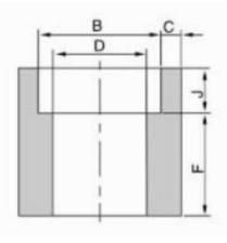
A182 F316 3000# Sw Half Pipe Fitting High Press Coupling
