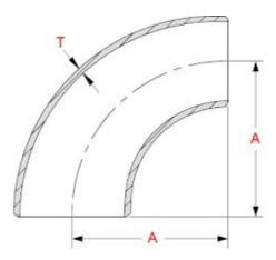
ANSI B16.9 Stainless Steel Special Pipe Fitting Elbow
