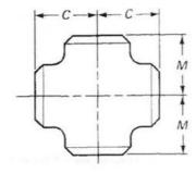
High Press Stainless Steel NPT Pipe Fitting Cross
