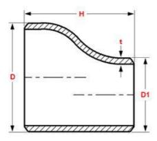
A234 WPB Carbon Steel Threaded Eccentric Special Pipe Fitting Reducer
