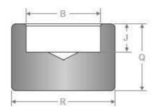
ANSI B16.11 High Press CL6000 Socket Weld Fittings Cap
