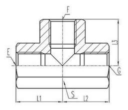
A234 Wpb Seamless Carbon Steel Large-Caliber Pipe Fitting Tee
