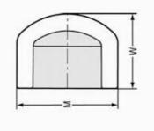
ASTM A234 Wpb Special Pipe fitting Caps
