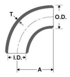
Welded Pipe Fitting Carbon Steel Large-Caliber Elbow
