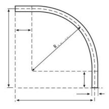
ASME B16.47 Schedule 80 10D Carbon Steel Special Pipe Fitting Bend
