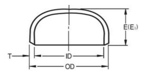
ASTM A234 Wpb Carbon Steel Large-caliber Pipe Fittings Cap
