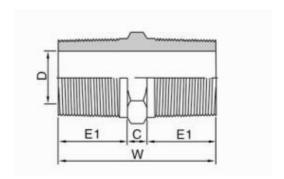
1/2" Stainless Steel Pipe Fitting Thread Screw Hex Nipple
