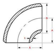
ASTM A234 Wpb Special Carbon Steel 90 Long Redius Elbow
