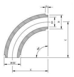
Stainless Steel 90 Degree 10D 304L Large-Caliber Pipe Fitting Bend
