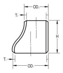
AISI Sch80 Carbon Steel Eccentric Special Pipeline Reducer
