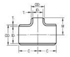
ASTM A234 Large-Caliber Carbon Steel Pipe Fitting Tee
