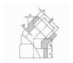
Sw Stainless Steel 45 Degree High Press Pipeline Elbow
