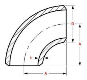
ASTM A403 WP304L Large Caliber Pipe Fitting Stainless Steel Elbow
