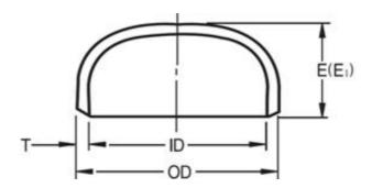
Large-Caliber ASTM Carbon Steel Pipe Fitting Cap
