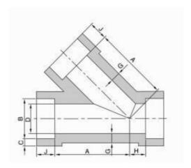
ASTM A234 WPB Carbon Steel 45 Degree Pipe Fitting Lateral Tee
