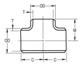
ANSI 316L Stainless Steel Customizable Seamless Pipe Fitting Tee
