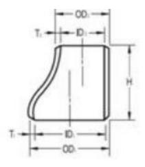
Large-Caliber Customized Stainless Steel Eccentric Reducer
