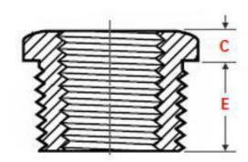
A182 Stainless Steel Forged Fitting Threaded Flush Bushing
