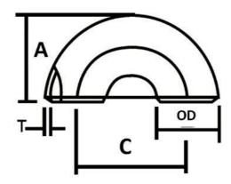
Large-Caliber ANSI B16.9 10D Seamless Carbon Steel Pipe Fitting Bend
