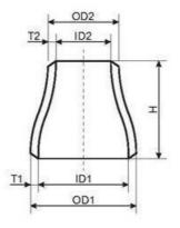
1/2" Butt Weld Eccentric Stainless Steel Reducer
