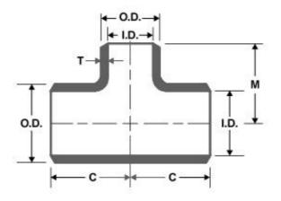
ASTM B16.9 Pipe Fitting Large-Caliber Stainless Steel Tee
