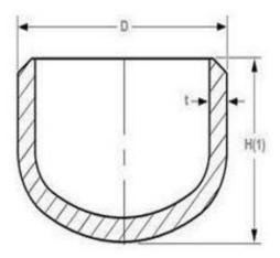
3/4" Special Stainless Steel Pipe Fitting Cap
