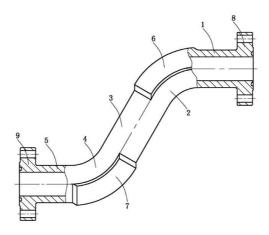
Stainless Steel S Shape Pipe Fitting Bend
