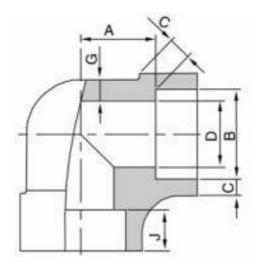
High Press ASME B 16.11 Socket Weld 90 Dergree Elbow
