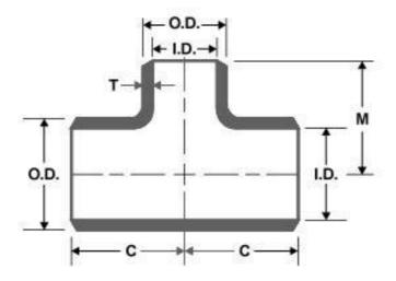
1/2" Small Caliber Carbon Steel Butt Welding Pipe Fitting Tee
