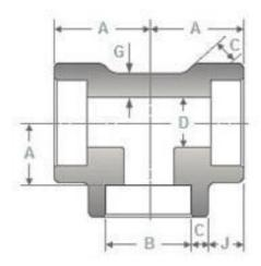
ASME B16.11 Alloy Steel A182 F11 Socket Weld Fitting Tee
