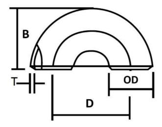
Large-Caliber Carbon Steel Pipe Fitting 90deg 10D Pipe Bend
