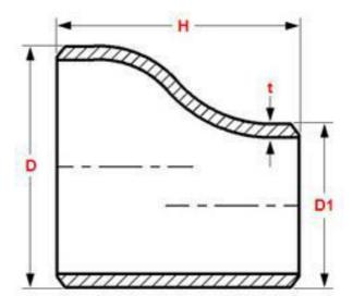
ASME B16.9 Eccentric Stainless Steel Pipe Fitting Reducer
