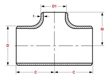
Large-Caliber Carbon Steel Butt Weld Seamless Pipe Fitting Tee
