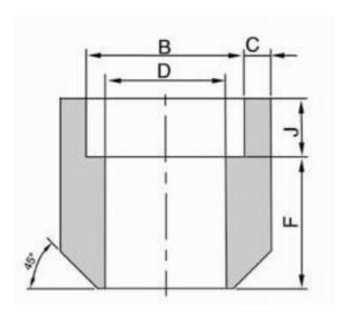
High press ASME B16.11 pipe fitting Boss
