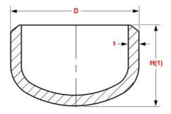
ASTM A234 Large-Caliber Carbon steel Pipe Fitting Cap
