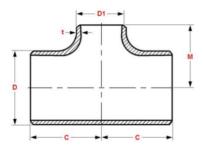
Large-caliber Carbon Steel Pipe Fitting Tee
